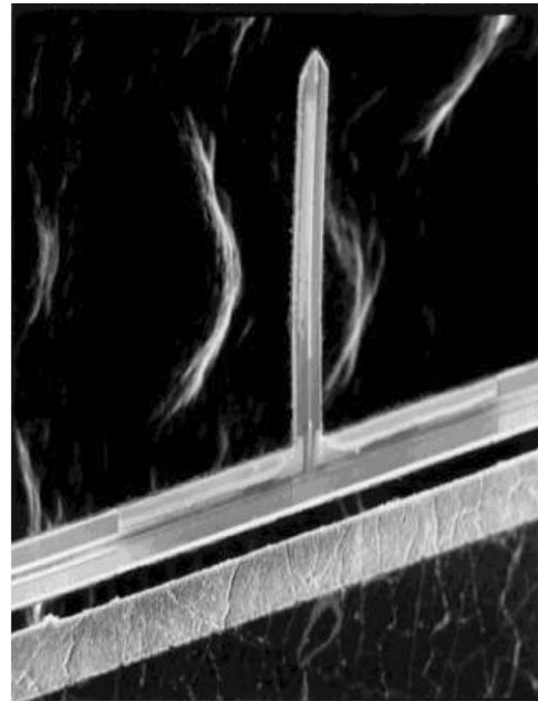
Fig. 2. Fabricated AFM cantilever with XYZ actuation by PZT thin film layer.
